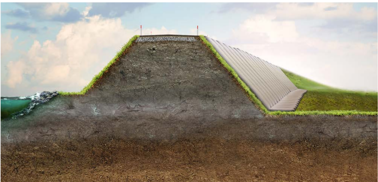
Figure 2: Tube mat as one-sided application on the air side of the dyke
