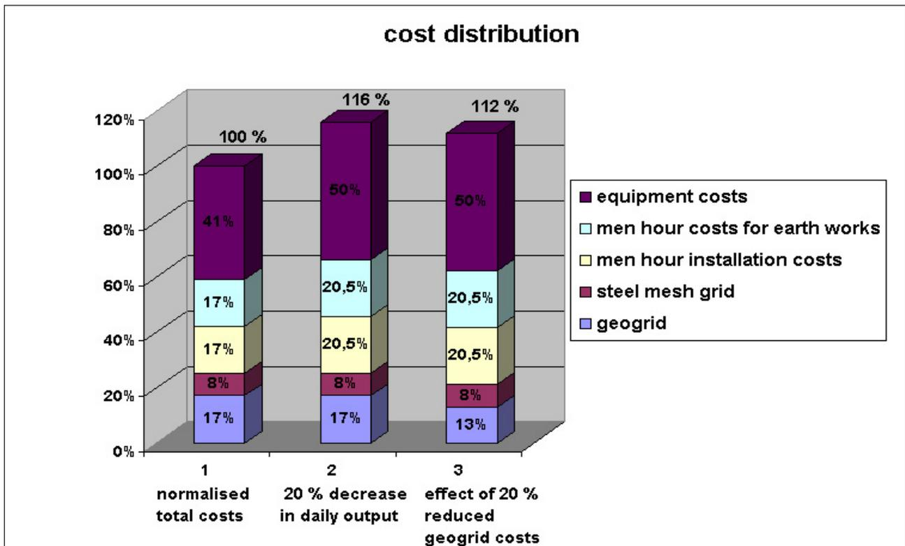
Fig. 3. Standardised total costs of a geosynthetic reinforced soil structure per m<sup>2</sup> of face area
