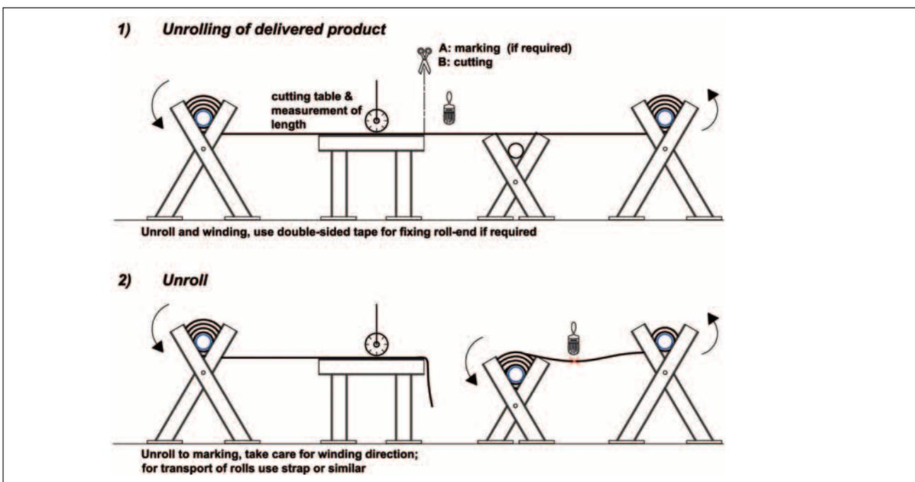
Fig. 12. principle of unrolling and winding station
