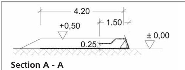
Fig. 6. Cross-section A-A through the "Steep reinforced soil slope" field test earthworks
