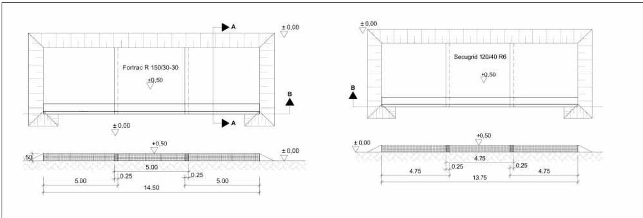
Fig. 4. Plan and longitudinal section of the trial earthworks for the “Steep reinforced soil slope” field test, left: Area 1 with flexible geogrid type 1, right: Area 2 with interlaced geogrid type 2.
