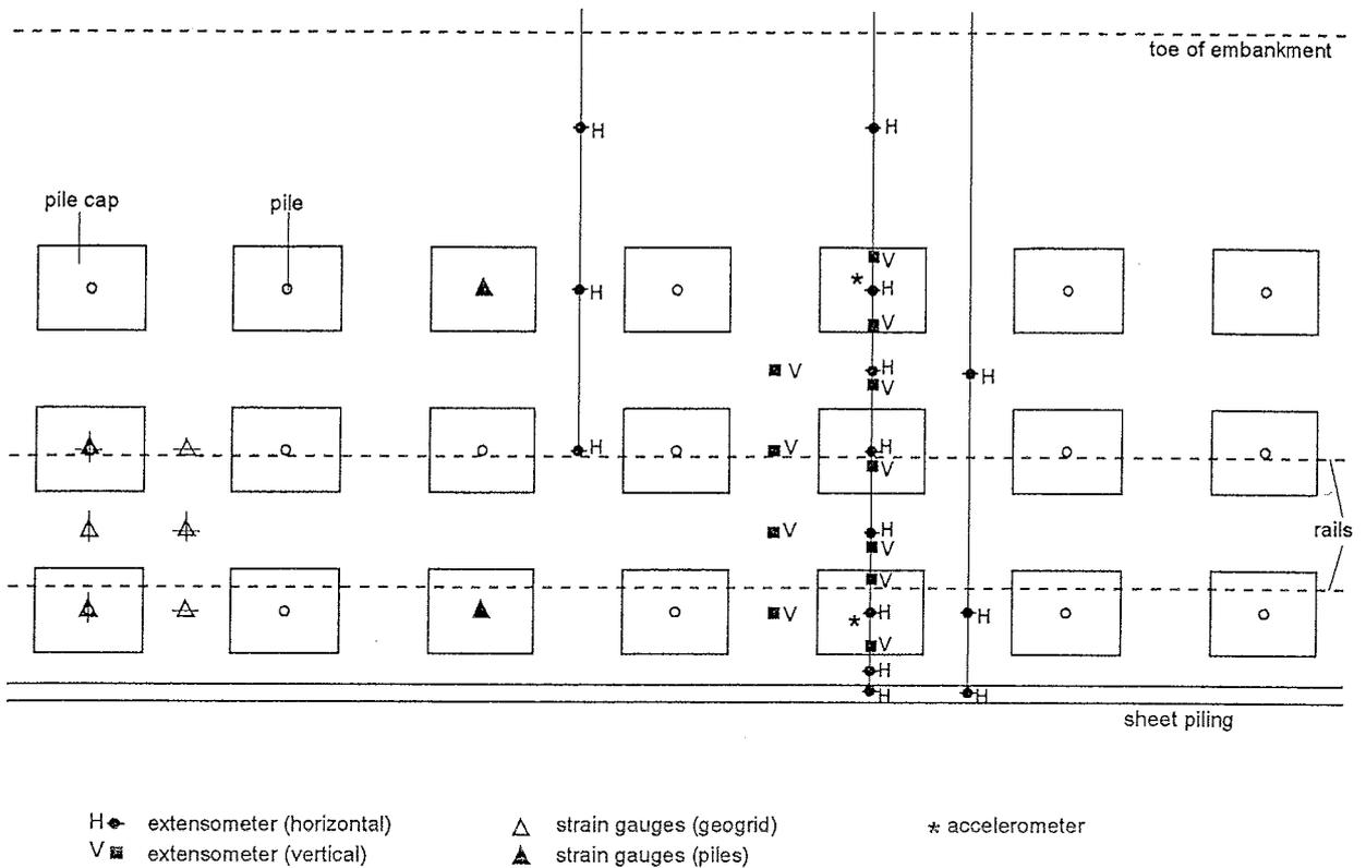
Fig. 2: Instrumentation of the monitoring section
