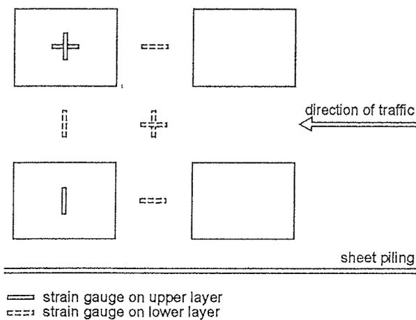
Fig. 3: Arrangement of strain gauges on geogrids
