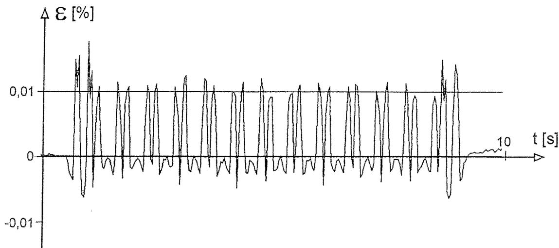
Fig. 9: Dynamic geogrid strains parallel to the embankment axis below train load
