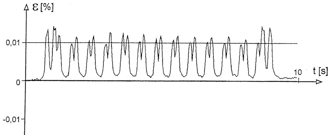
Fig. 8: Dynamic geogrid strains perpendicular to the embankment axis below train load
