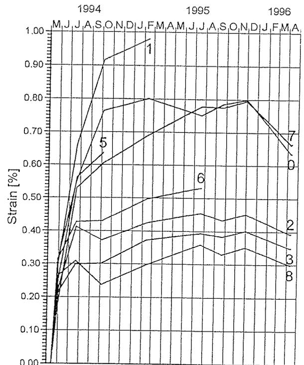
Fig. 7: Static geogrid strains with time
