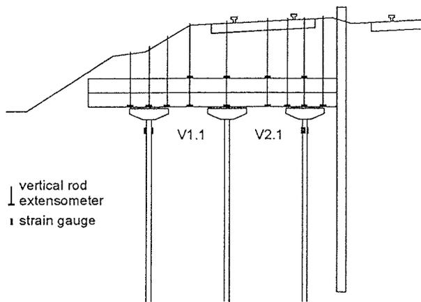
Fig. 4: Vertical rod extensometers
