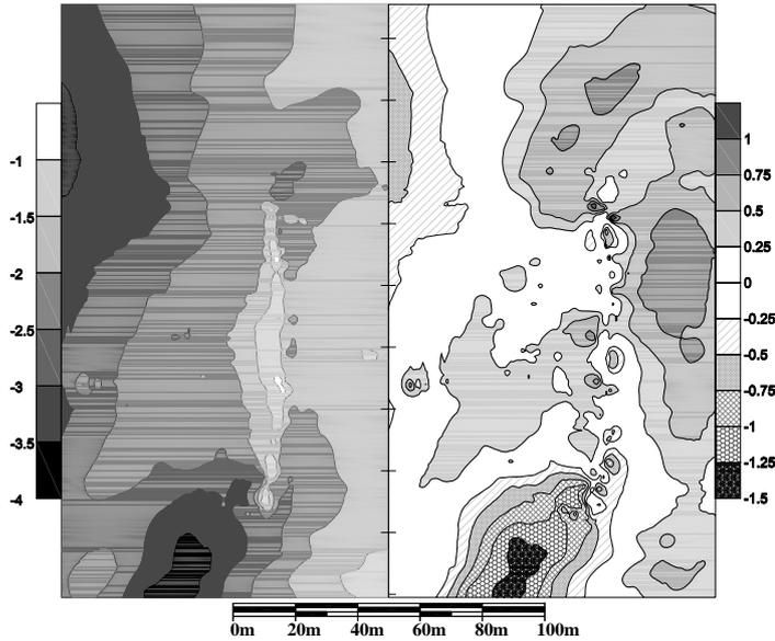
Figure 11 Bathymetry obtained a few months after construction of defence system (18 November 2008) (left); Comparison of bathymetry surveyed in two occasions after installation: 28 August and 18 November 2008 (right).
