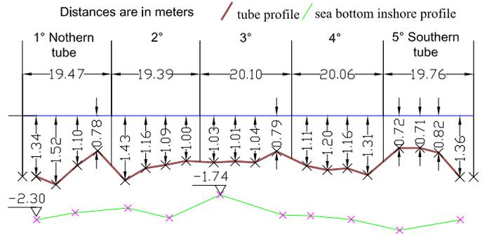
Figure 9 Longitudinal section of the barrier after consolidation (August 2008)
