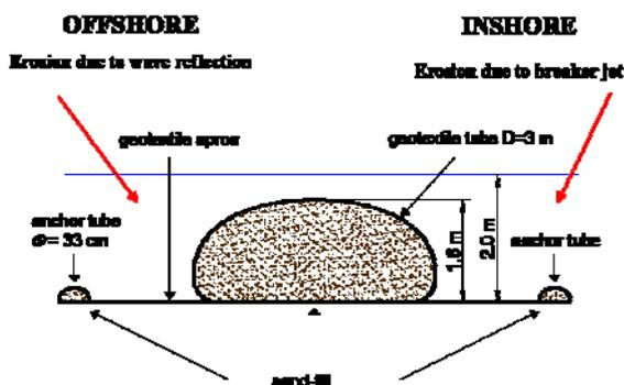
Figure 3 Section of tube and scour apron
