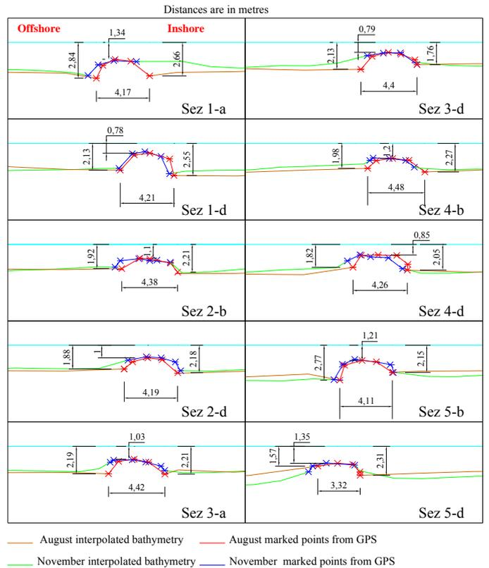
Figure 10 Geometrical evolution of the tube and surrounding sea-bottom - quotes are referred to the first survey.
