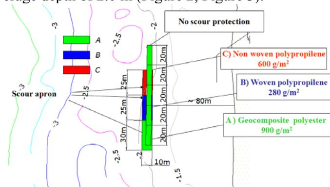
Figure 2 Outline of tubes placement and materials employed
