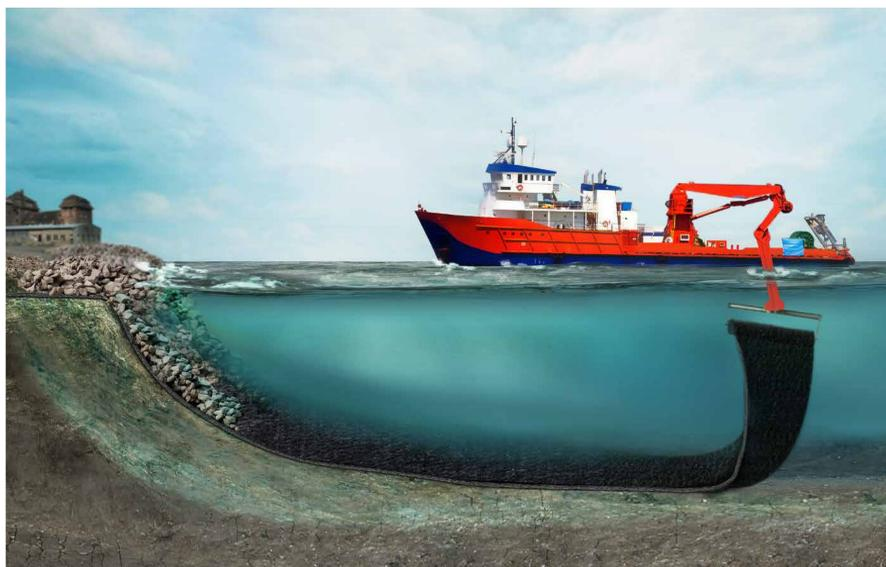
**Active Geo-Composites** consist of an amendment, or multiple amendments, sandwiched between two geosynthetic layers. These Geo-Composites allow accurate placement of amendments with low densities that could otherwise become suspended during placement.
