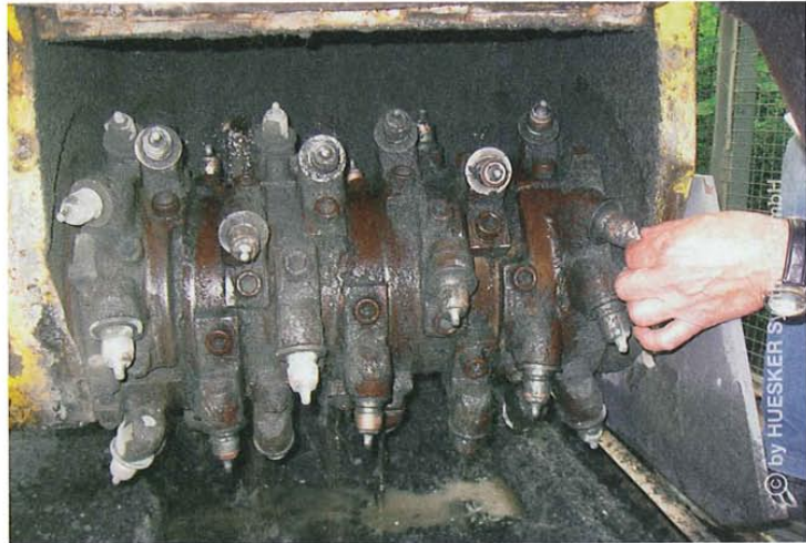
Virtually no fibres remained on the milling drum
